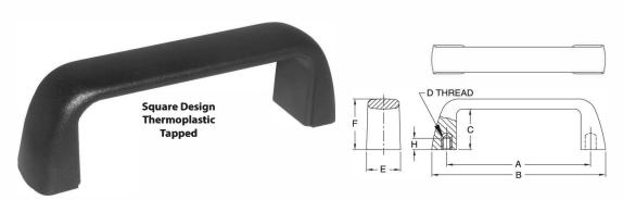
Attractive, modern-design handle that provides a comfortable grip with good ergonomic features. Excellent durability. Textured non-slip, non-glare finish. Molded-in brass insert provides superior thread strength. Black fiber-reinforced nylon thermoplastic (textured surface for secure gripping, excellent impact resistance, operating temperatures to 230°F). Choice of two handle sizes, available with either inch or metric threads.
